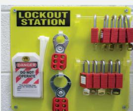
Ensure you have the proper tools to properly perform a lockout-tagout
