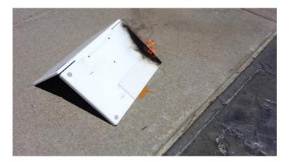
We have since determined that the overheating was most likely caused by an aftermarket battery used in that model laptop. The aftermarket battery was necessary because the laptop was eight years old, and Apple no longer manufactures stock replacement batteries for that old of a machine.
